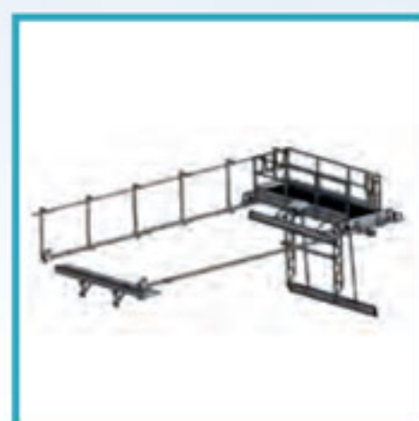
PVV Carroponte va e vieni "Come and go" scraping bridge
